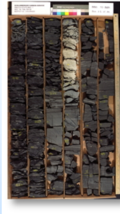
1 of 7 boxes of slabbed core from the RMCCS well
